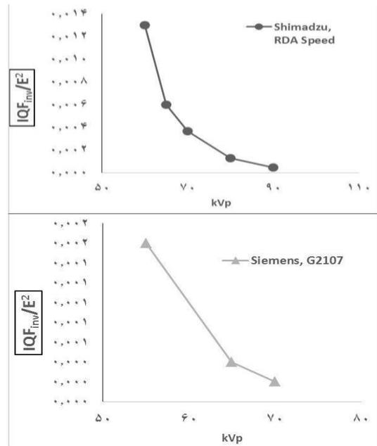
**Figure 5.  $IQF_{inv}/E^2$  in terms of kVp for Shimadzu RDA Speed (source to detector distance=150 cm) and for Siemens G2107 (source to detector distance=110 cm)**
