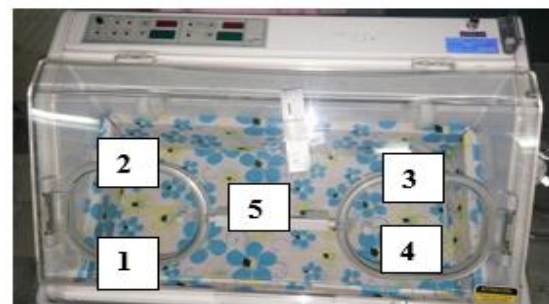
Figure 1. The points used inside the incubator to measure the magnetic field intensity
