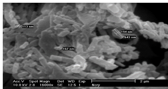
Figure 1. Chrysin nanoparticle image by electron microscope (SEM)
