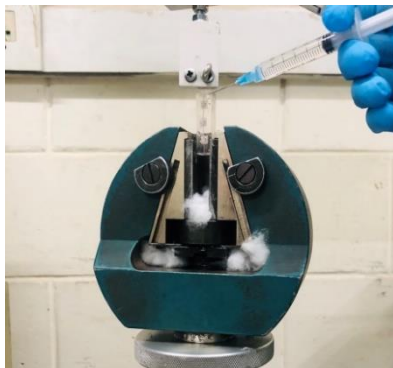
Figure 2. A friction test using the Instron machine, with artificial saliva dripping from a plastic syringe during the test
