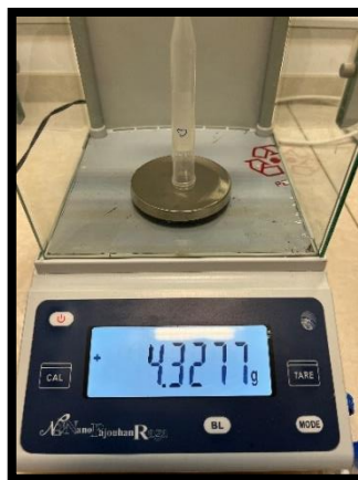
Figure 1. Weighing uncapped tubes on a scale with an accuracy of 0.0001 g
